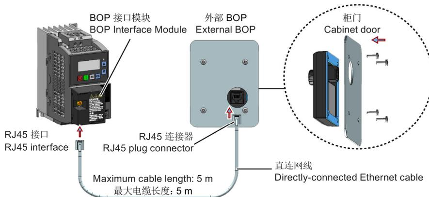
To meet EMC requirements, you must use a directly-connected shielded Ethernet cable, with a maximum length of 3 m.
