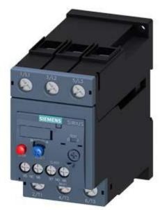
OVERLOAD RELAY 54...65 A FOR MOTOR PROTECTION SIZE S2, CLASS 10 STAND-ALONE INSTALLATION MAIN CIRCUIT: SCREW TERMINAL MANUAL-AUTOMATIC-RESET.
