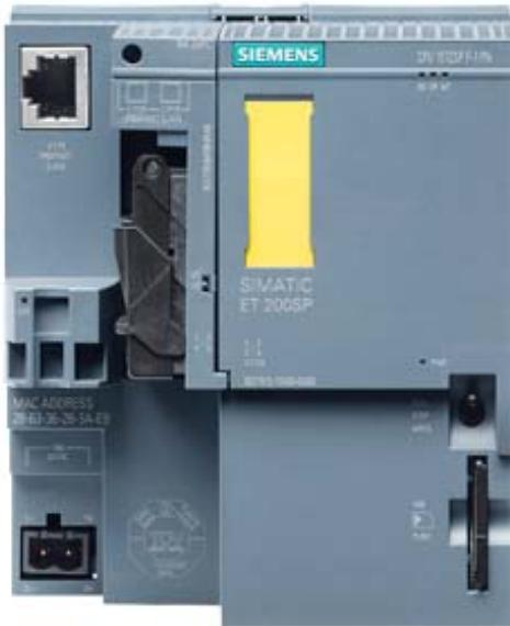
SIMATIC DP, CPU 1512SP F-1 PN FOR ET 200SP, CENTRAL PROCESSING UNIT WITH WORKING MEMORY 300 KB FOR PROGRAM AND 1 MB FOR DATA, 1. INTERFACE: PROFINET IRT WITH 3 PORT SWITCH, 48 NS BIT-PERFORMANCE, SIMATIC MEMORY CARD NECESSARY, BUSADAPTER NECESSARY FOR PORT 1 AND 2
