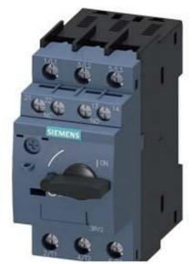
CIRCUIT-BREAKER SZ S0, FOR MOTOR PROTECTION, CLASS 10, A-REL.2.2...3.2A, N-REL. 42A SCREW CONNECTION, STANDARD SW. CAPACITY W. TRANSVERSE AUX. SWITCH 1NO+1NC
