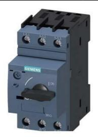
CIRCUIT-BREAKER SZ S0, FOR MOTOR PROTECTION, CLASS 10, A-REL. 4.5...6.3A, N-REL. 82A SCREW CONNECTION, STANDARD SW. CAPACITY
