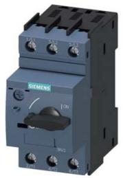
CIRCUIT-BREAKER SZ S00, FOR MOTOR PROTECTION, CLASS 10, A-REL. 0.55...0.8A, N-RELEASE10 A SCREW CONNECTION, STANDARD SW. CAPACITY
