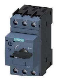
CIRCUIT-BREAKER SZ S0, FOR MOTOR PROTECTION, CLASS 10, A-REL.2.2...3.2A, N-REL. 42A SCREW CONNECTION, STANDARD SW. CAPACITY
