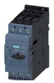
CIRCUIT BREAKER, SIZE S2, FOR MOTOR PROTECTION, CLASS 10, A-RELEASE 35...45A, N-RELEASE 650A, SCREW TERMINAL, INCREASED SWITCHING CAPACITY
