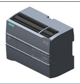
SIMATIC S7-1200, CPU 1215C, COMPACT CPU, DC/DC/RELAY, 2 PROFINET PORT, ONBOARD I/O: 14 DI 24V DC; 10 DO RELAY 2A, 2 AI 0-10V DC, 2 AO 0-20MA DC, POWER SUPPLY: DC 20.4 -28.8 V DC, PROGRAM/DATA MEMORY: 125 KB
