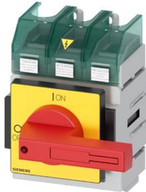
SENTRON 3LD5 switch disconnector UL, EMERGENCY-OFF switch, 3-pole, approved according to UL 489, UL 60947-4-1 and IEC 60947-3, UL: 100 A, SCCR 65 kA at 480 V AC, operational power @ 480 V AC 3-phase: 60 hp, IEC: 100 A, operational power at AC-23 A at 400 V: 45 kW, floor mounting with direct operating mechanism, red/yellow including terminal covers for the infeed side
