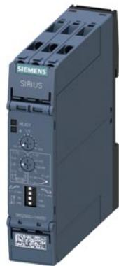
temperature monitoring relay Pt100, thermocouple J, K 1 threshold value, width 22.5 mm overshoot and undershoot 24 - 240 V AC/DC 1 change-over contact, quiescent current principle screw terminal
