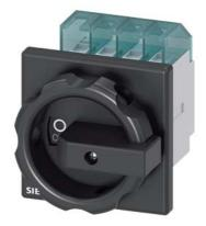
SENTRON, Switch disconnector 3LD, main switch, 4-pole, lu: 16 A, Operating power / at AC-23 A at 400 V: 7.5 kW, front-mounted, rotary operating mechanism, black, 4-hole mounting of the handle
