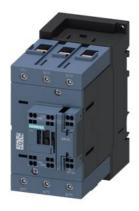
power contactor, AC-3e/AC-3, 80 A, 37 kW / 400 V, 3-pole, 24 V AC, 50 Hz, auxiliary contacts: 1 NO + 1 NC, main circuit: screw terminal, control and auxiliary circuit: spring-loaded terminal, size: S3  $\,$
