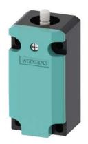
Position switch Basic switch Metal, 40 mm, according to EN 50041 Increased corrosion protection Device connection 1 x (M20 x 1.5) 1 NO/1 NC quick action contacts functional at -40  $^{\circ}\text{C}$  Shock and vibration test according to EN 61373, Category 1B
