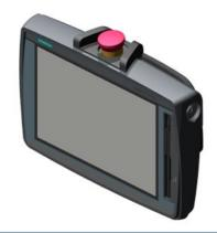
SIMATIC HMI TP1000F MOBILE 10.0" TFT display, 1280x800 pixels, 16 million colors, Touch operation, touch pen, 1x PROFINET/Industrial Ethernet interface, 1x multimedia card, 1x USB, key-operated switch, acknowledgement button, 1 emergency stop/stop button confiigurable from WinCC Comfort V14
