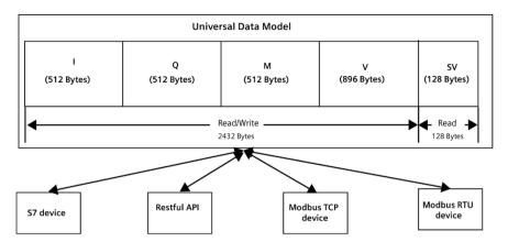
I, Q, M, V constructed a data model to simulate the process image in PLC.
