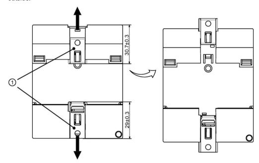
2. Feed the screws through the openings in the catches and secure the device to the wall.
