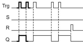
The bold printed section of the timing diagram is also shown in the symbol for the pulse relay.
