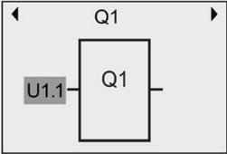
5. Press **OK** and the cursor appears in a flashing solid square. Select an empty input by pressing **▲** or **▼**. Press **OK** and LOGO! shows the following display:
