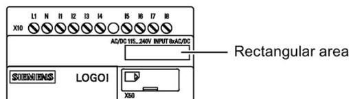
In the case of expansion modules, you can use the rectangular areas for labeling the inputs and outputs, for example. In this connection, you can enter a delta factor of +8 for the inputs or +4 for the outputs if the LOGO! Base Module already has 8 inputs or 4 outputs.
