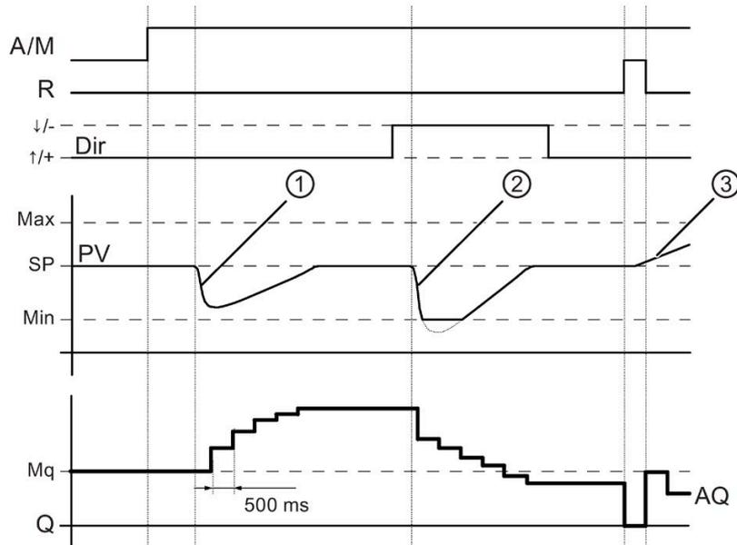
1. A disturbance causes the PV to drop, as Dir is positioned upwards, AQ increases until PV corresponds again to SP.
