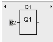
9. Now set the blank connector at output Q1 instead of block B2:
