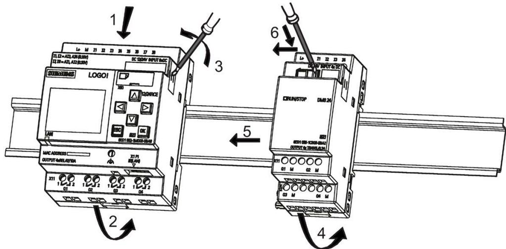
3. On the right side of the LOGO! Base Module/LOGO! expansion module, remove the connector cap.
