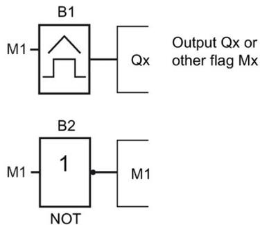
2. Configure the threshold trigger as shown below. LOGO! generates a pulse in each program cycle due to the inverted flag. The trigger interval is 2 seconds.
