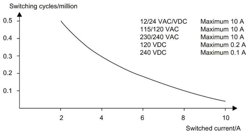
**Switching capacity and service life of the contacts with high inductive load to IEC 60947-5-1 DC 13/AC 15 (contactors, solenoid coils, motors):**
