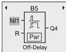
You can see that there is a network digital input NI1 connected at the first input of B5. The following views are examples of network digital and analog outputs in LOGO!:
