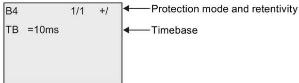
To change the timebase, press **▶** to move the cursor to "10ms". Press **OK** and now the timebase can be selected. Press **▲** or **▼** to select another timebase. To confirm your selection, press **OK**.
