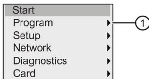
The first line is highlighted. Press ▲ and ▼ to move the highlight bar up and down. Move it to "①" and confirm with **OK**. LOGO! opens the programming menu.
