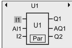
1. Press **▼** to move the cursor to "Par" and press **OK**. LOGO! shows you the following display (T and TH are the identifiers you specified for the relevant UDF parameters in LOGO!Soft Comfort . You can configure a maximum of eight parameters for each UDF block using LOGO!Soft Comfort. LOGO! can show a maximum of three parameters on a single display.):
