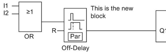
You can see the OR block and the output relay Q1 that you used in the first circuit program. The only difference is the new off-delay block.
