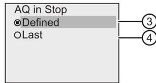
The circle with a dot before "④" above indicates the current setting for the analog output channels.
