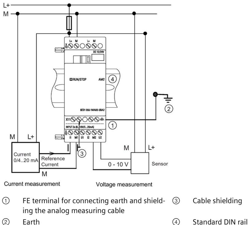
The illustration above shows an example of four-wire current measurement and two-wire voltage measurement.
