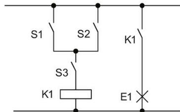
The switches (S1 OR S2) AND S3 activate the relay K1 and switch on the load at E1.
