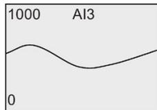
The display refreshes continuously and the curve shifts to the left of the display bit by bit. You can press ◀ or ▶ to move the screen form to the left/right in order to view the earlier/later value changes.
