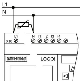
To suppress surge voltages, install varistors (MOV) with an operating voltage at least 20% above the rated voltage.
