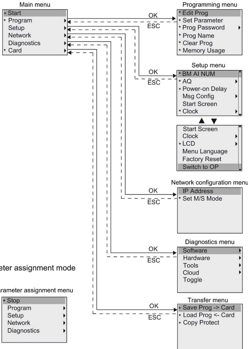
Note: The "BM AI NUM" selection is only available on Base Modules that support four analog inputs.
