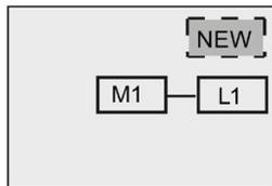
2. Move the cursor to "L1" by pressing ▼ (The data log is identified with a "L1"). Press **OK**. LOGO! shows the following display:
