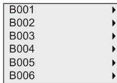
If no parameter can be set, the display shows as follows, and you can press **ESC** to return to the parameter assignment menu.
