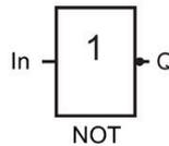
The output status is 1 if the input is 0. The NOT block inverts the input status.
