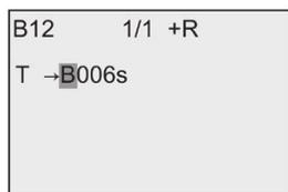
3. Press ► to move the cursor to the "B" of the shown block, and then press ▼ to select the required block number.
