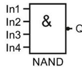
The output of the NAND is only 0 if the status at **all** inputs is 1, that is, the contacts are closed.
