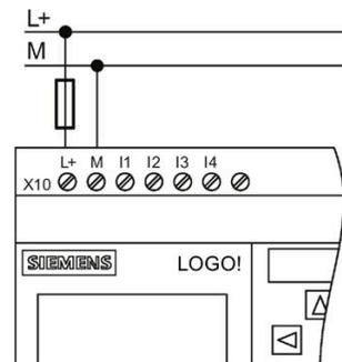
Protection with safety fuse if required (recommended) for:
