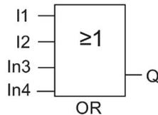
Inputs I1 and I2 connect to the OR block. The last two inputs of the block remain unused.
