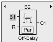
LOGO! automatically connects the uppermost input of the new block to B1, which you had previously connected to Q1. Note that you can only interconnect digital inputs with digital outputs or analog inputs with analog outputs. LOGO! otherwise removes the 'old' block.
