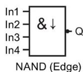
The output status of the NAND with edge evaluation is only 1 if **at least one** input is 0 and if **all** inputs were 1 in the previous cycle.
