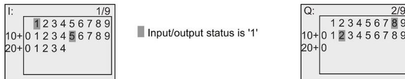
In this example, only the inputs I1 and I15 and the outputs Q8 and Q12 are set "high".
