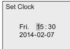
8. To set the correct time of day, press ◀ or ▶ to move the cursor to the desired position, and press ▲ or ▼ to change the value.
