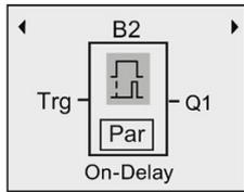
When you select a special or basic function block, LOGO! shows you the relevant function block and positions the solid square cursor on the block. Press **OK** to enter the editing mode, and the cursor appears as a flashing solid square. Press ▲ or ▼ to select the required block.
