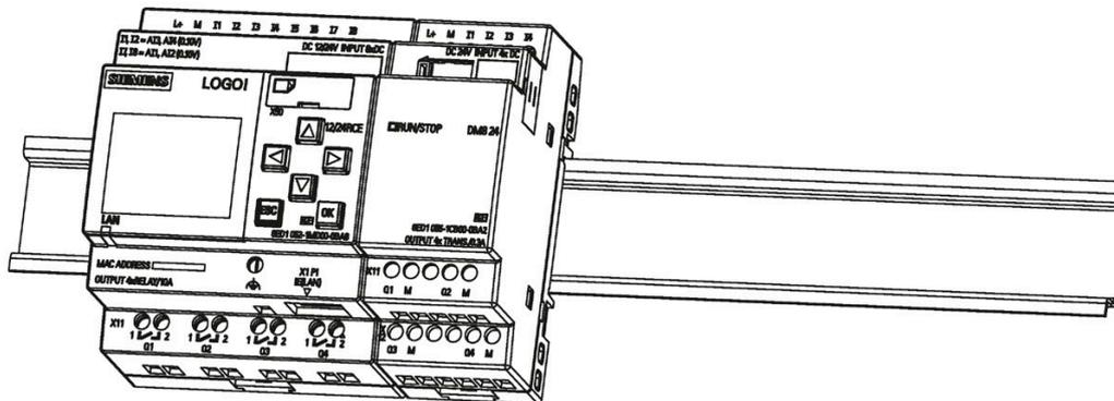
Repeat the digital module steps to mount further expansion modules.
