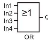
The output status of the OR element is only 1 if **at least one** input is 1, that is, at least one of the contacts is closed.
