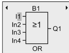
Press **OK** to confirm. You have now connected I1 to the input of the OR block.
