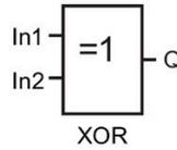
The output status of the XOR is 1 if the inputs are **not equivalent**.
