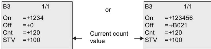
You can change the on/off threshold. This does not apply if the on or off threshold represents the result of another function (In the "Up/down counter (Page 180)" topic, this is B021).
