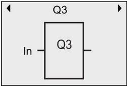
2. Move the cursor to "In" by pressing **◀**. Press **OK** and the cursor appears in a flashing solid square. You can change the input to "U1.1" ("1" refers to the first output of the UDF block that is connected to "Q1") by pressing **▲** or **▼** and LOGO! shows the following display:
