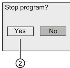
4. Confirm placing LOGO! in STOP mode by pressing **OK** with the cursor on "②".
