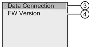
5. You can select "③" to view the real-time status of the S7 connection or Modbus connection. Select "④" to view the firmware version of LOGO!.
