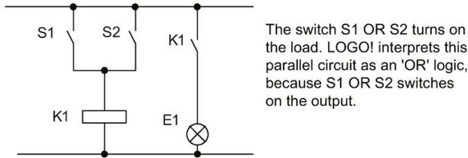
The switch S1 OR S2 turns on the load. LOGO! interprets this parallel circuit as an 'OR' logic, because S1 OR S2 switches on the output.
