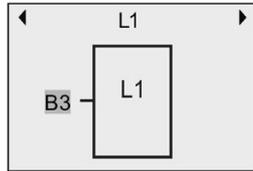
4. In the following example, you can see that this "L1" is now connected to the B3 block:
