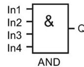
The output of the AND is only 1 if **all** inputs are 1, that is, all contacts are closed.
