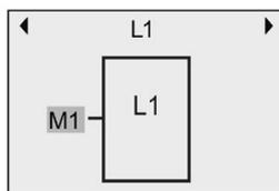
3. Press **OK** on the selected input ("M1" in this example) and the cursor appears in a flashing solid square. To select a different element from the available list (for example, B3), press **▼**. Press **OK**. LOGO! shows the following display:
