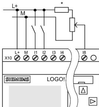
The inputs of these devices are not isolated and therefore require a common reference potential (chassis ground).
