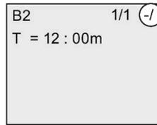
When the protection mode shows "+", you can modify the time T in parameter assignment mode.
