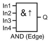
The output of an edge-triggered AND is only 1 if **all** inputs are 1 and if **at least one** input was low in the previous cycle.
