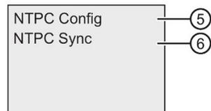
To enable NTP Client function, press ▲ or ▼ to select "⑤";
