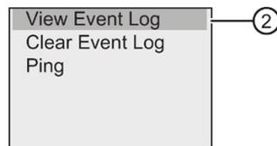
4. Confirm "②": Press **OK**. LOGO! displays all errors detected. You can press **◀** or **▶** to view each error record. Press **ESC** or **OK** to return to the previous menus.
