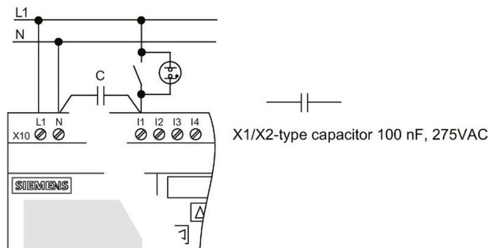
Take into account the quiescent current of any two-wire proximity switches that you use. The level of the quiescent current of some two-wire proximity switches is high enough to trigger a logical "1" signal at the LOGO! input. You should therefore compare the quiescent current of the proximity switches with the technical data of inputs (Page 324).
