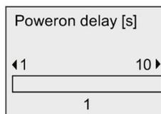
5. Press **▶** or **◀** to increase or decrease the delay time by 0.2 s. You can also press and hold down **▶** or **◀** to quickly increase or decrease the time.
