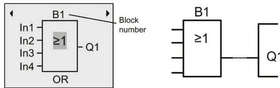
You have now entered the first block. LOGO! automatically assigns a block number to each new block. If you assign a name to the block, LOGO! shows the block name instead of the block number. You can assign a block name as required:
