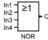
The output status of the NOR is only 1 if **all** inputs are 0, that is, off. The NOR output is set to 0 when one of the inputs is on (logical 1 status).
