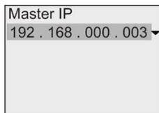
7. In this view, you enter the IP address of the LOGO! that you want to configure to be the master of your slave LOGO!. To change the setting, press **OK**. When the cursor appears in a flashing solid square, press ◀ or ▶ to move the cursor through the numbers. Press ▲ or ▼ to change the number.
