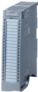
SIMATIC S7-1500, analog input module AI 16xU BA, 16-bit resolution accuracy 0.5%, 16 channels in groups of 16, common mode voltage 4 V DC, diagnostics, hardware interrupts; delivery including infeed element, shield bracket and shield terminal: front connector (screw terminals or push-in) to be ordered separately
