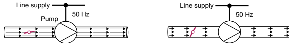
Figure 8-83 Flow control with pump and throttle connected to a 50 Hz line supply
