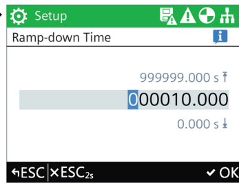
Enter required Ramp-down Time
