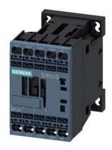
Power contactor, AC-3 7 A, 3 kW / 400 V 1 NC, 110 V AC, 50 / 60 Hz 3-pole, Size S00 Spring-type terminal
