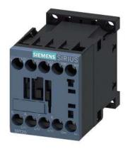
Power contactor, AC-3 7 A, 3 kW / 400 V 1 NC, 110 V DC 3-pole, Size S00 screw terminal
