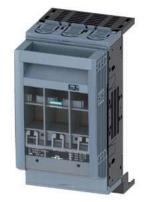
SENTRON, Fuse switch disconnector 3NP1, 3-pole, NH00, 160 A, for Rittal busbar system 60 mm, flat terminal, Cover level 32/70 mm
