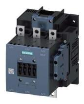
Power contactor, AC-3 185 A, 90 kW / 400 V AC (50-60 Hz) / DC operation 23-26 V UC Auxiliary contacts 2 NO + 2 NC 3-pole, Size S6 Busbar connections Drive: conventional screw terminal
