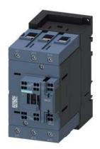
Power contactor, AC-3 110 A, 55 kW / 400 V 1 NO + 1 NC, 230 V AC, 50 Hz 3-pole, 3 NO, Size S3 Spring-type terminal
