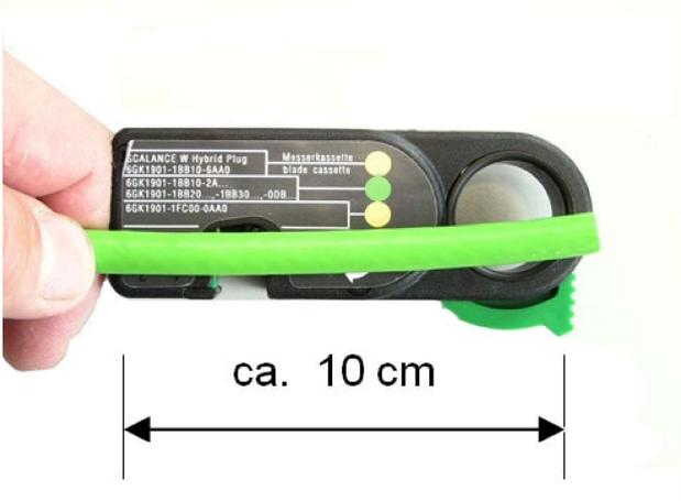
3. Place the cable in the stripping tool. Make sure that a length of approximately 10 cm is stripped.
