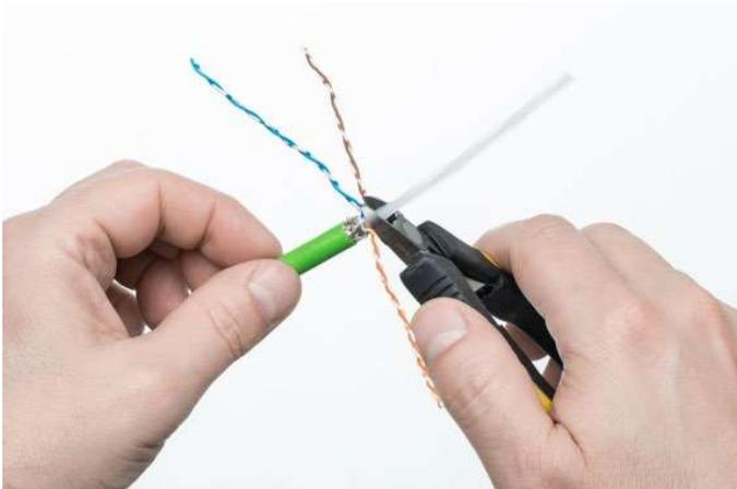
9. Release the wires and pull them parallel. Make sure that the ends are not crushed. Sometimes it is necessary to trim the ends.
