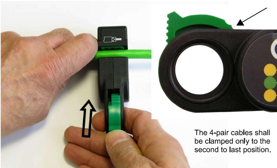
The 4-pair cables shall be clamped only to the second to last position.
