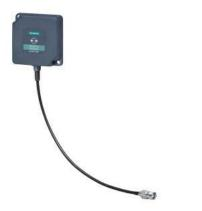
SIMATIC RF600 antenna RF622A; ETSI frequency 865-868 EU linear IP67, -20 to +70  $^{\circ}\text{C}$ , with 30 cm connecting cable
