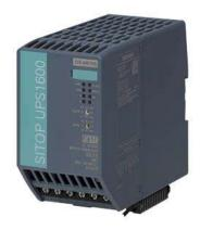
SITOP UPS1600 40 A Ethernet/ PROFINET Uninterrupted Power supply with Ethernet/ PROFINET interface / OPC UA Server / Web server input: 24 V DC output: 24 V DC/40 A
