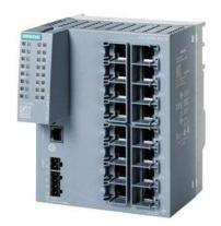
SCALANCE XC216 managed Layer 2 IE switch; IEC 62443-4-2 certified; 16x 10/100 Mbps RJ45 ports; 1x console port, diagnostics LED; redundant power supply; temp. range -40 °C to +70 °C; mounting: DIN rail/S7 mounting rail/wall Office redundancy functions features (RSTP, VLAN,...); PROFINET IO device; Ethernet/IP-compliant; C-plug slot;
