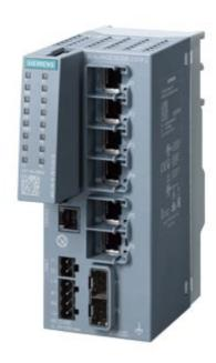
SCALANCE XC206-2SFP G Manageable layer 2 IE switch; 6x 10/100/1000 Mbit/s RJ45 ports; 2x 1000 Mbit/s SFP; 1x console port; Diagnostics LED; Redundant power supply; Temp. range -40 °C to +70 °C Mounting: Standard mounting rail/S7 mounting rail/wall; Redundancy functions; Office features (RSTP, VLAN,...); PROFINET IO device; Ethernet/IP-compliant; C-PLUG slot;
