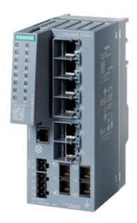
SCALANCE XC206-2 manageable layer 2 IE Switch; 6x 10/100 Mbit/s RJ45 ports; 2x 100 Mbit/s SC ports; 1x console port; Diagnostic LED; Redundant power supply; Temp. range -40°C to +70 °C Mounting: Standard Mounting Rail/S7 Profile Rail/Wall; redundancy functions; office features (RSTP, VLAN ,...); PROFINET IO device Ethernet/IP-compliant C-PLUG shaft
