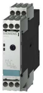
Timing relay, electronic Phased-out product !!! For further information, please contact our sales department OFF delay 1 change-over contact, with auxiliary voltage 1 time range, 5 s...100 s 24 AC, 100...127 V and 24 V DC at 50/60 Hz AC with LED, Screw terminal
