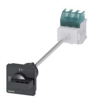
SENTRON, switch disconnector 3LD, main switch, 3-pole, Iu: 32 A, operating power / at AC-23 A at 400 V: 11.5 kW, floor mounting with door coupling, defeatable knob-operated mechanism, black, 4-hole mounting of the handle
