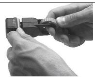
4. Fit the measured end of the cable into the stripping tool as far as allowed by the index finger of your left hand.
