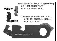
1. Fit the required knife cassette in the stripping tool. If your stripping tool was supplied with a yellow knife cassette, the cutting depth must be adjusted with the middle socket-head screw after fitting the new cassette!
