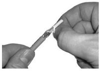
9. If the white filler was not removed during stripping, pull this off with your hand.
