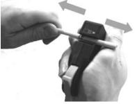
7. Keeping the stripping tool closed, pull it off the end of the cable along with the jacket and remnants of the shield.
