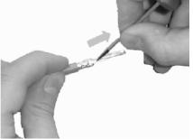
10. The protective foil is easier to remove if you score it between the wires with a screwdriver.
