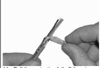
11. Pull the protective foil off the wires
