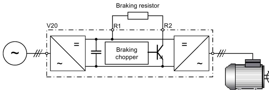
The continuous power  $P_{DB}$  and the duty cycle for the braking resistor can be modified using the dynamic braking module (for frame size A / B / C) or parameter P1237 (for frame size D).
