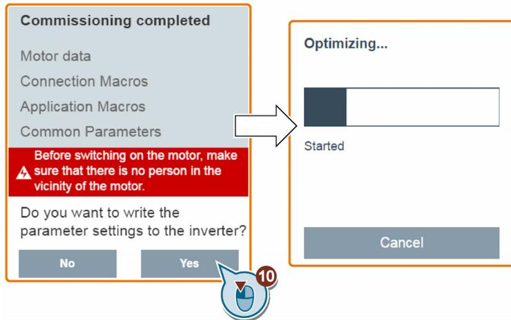
8. Confirm completion of the quick commissioning when the following window appears. If the Web page indicates that the optimization fails, you can select to try optimization again.
