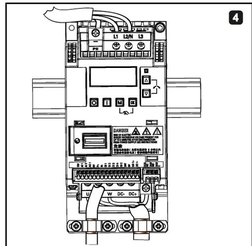
Removing FSA from the DIN rail
