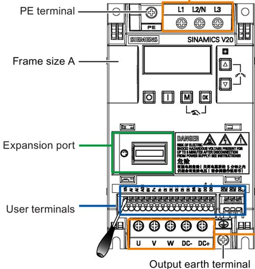
Align a flat-bit screwdriver (bit size: 0.4 x 2.5 mm) with the terminal. Push it downwards on the release lever with a maximum force of 12 N and insert the control wire from below.
