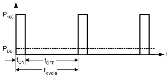
Dynamic braking switch-on level:
