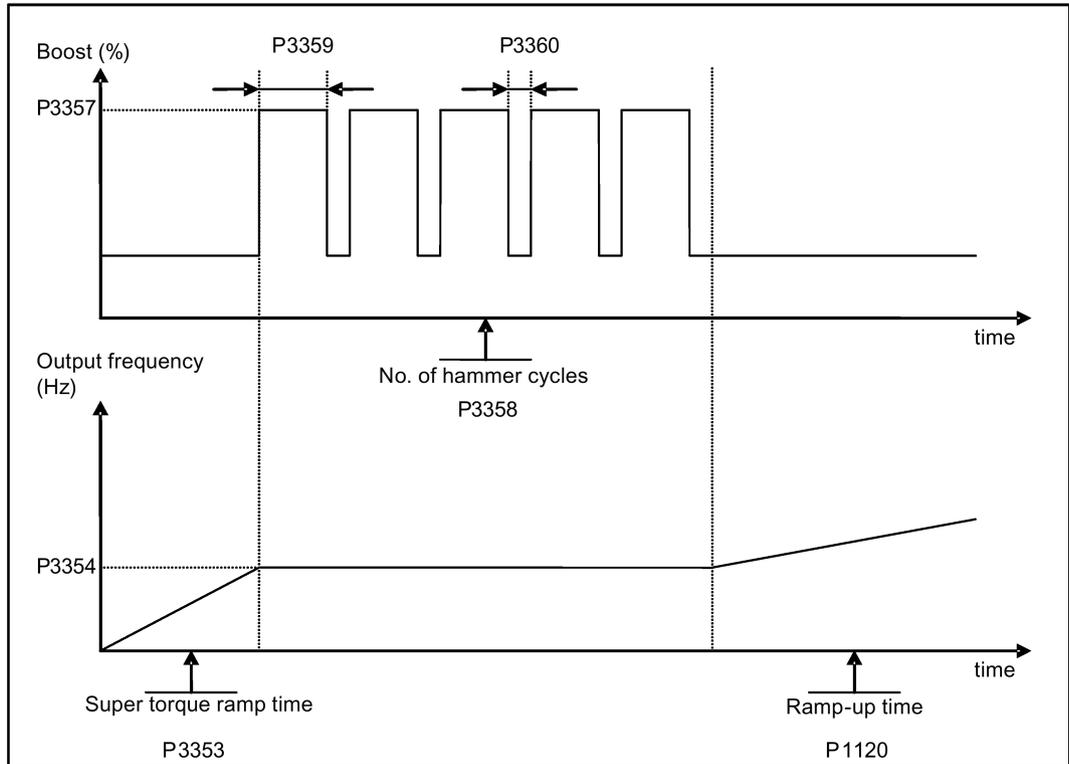
**5.6.3.3 Starting the motor in blockage clearing mode**
