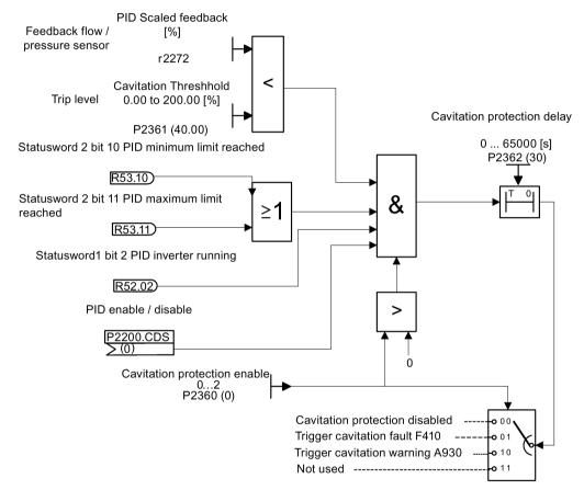
**Cavitation Protection Logic Diagram**
