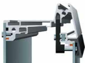
Front panel installation screwed from front
