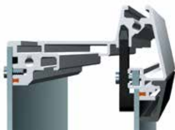
Front panel installation from rear
