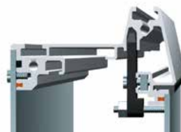
Front panel installation with stud bolts
