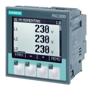
SENTRON, Measuring instrument, 7KM PAC3200, LCD, L-L: 500 V, L-N: 289 V, 5 A, Modbus TCP, optionally Modbus RTU / PROFINET / PROFIBUS, apparent / active / reactive energy, Class 0.5 acc. to IEC61557-12 or Class 0.5S acc. to IEC62053-22 ELV power supply unit, DC, screw terminal
