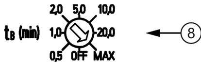
Figure 2-12 Rotary coding switch, buffer time
