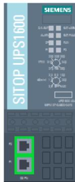
7. Under "Ethernet addresses" in the inspector window enter the IP address of the SITOP UPS1600, which was already assigned in the TIA Portal.
