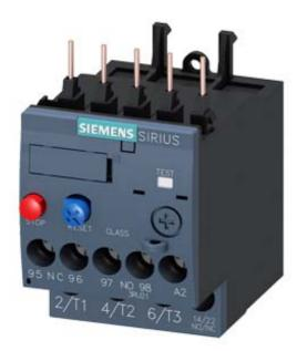
OVERLOAD RELAY 1.8...2.5 A FOR MOTOR PROTECTION SZ S00, CLASS 10, F. MOUNTING ONTO CONTACTOR MAIN CIRCUIT: SCREW TERMINAL AUX. CIRCUIT: SCREW TERMINAL MANUAL-AUTOMATIC-RESET
